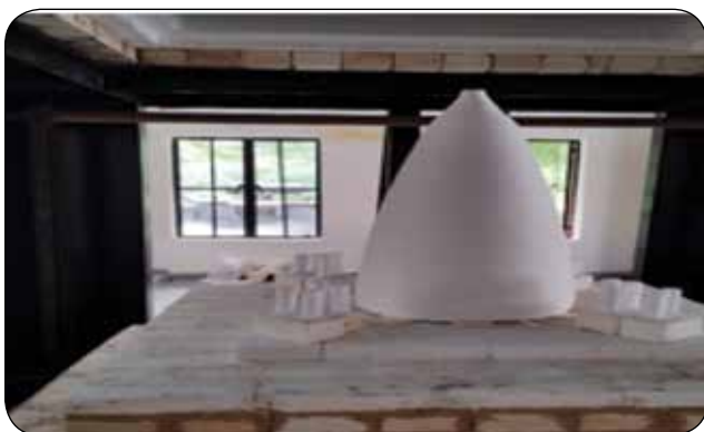
Bottom Loading Furnace Max.Temp.: 1300 °C Chamber Dimension: 1 X 1 X 1 m
