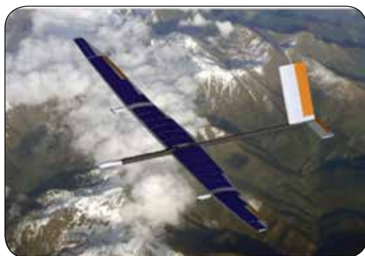
CAD rendering of the aircraft HAP SubScale Ver4.0
