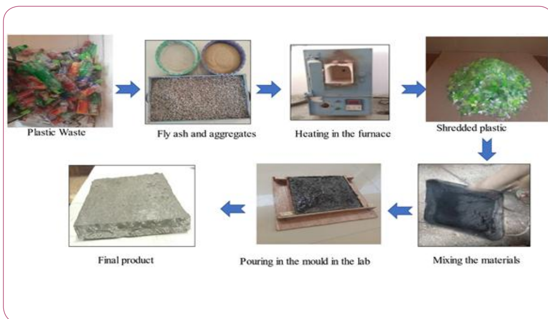
Steps for producing construction material by recycling the waste plastic
