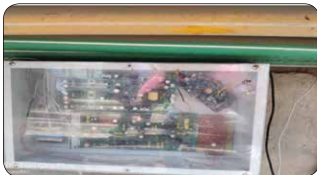
Prototype Broken Rail Detection System At ShaheenBagh
