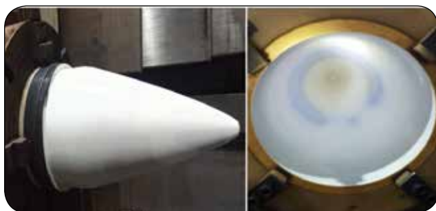
Outer profile machining in progress Inner profile machining in progress
